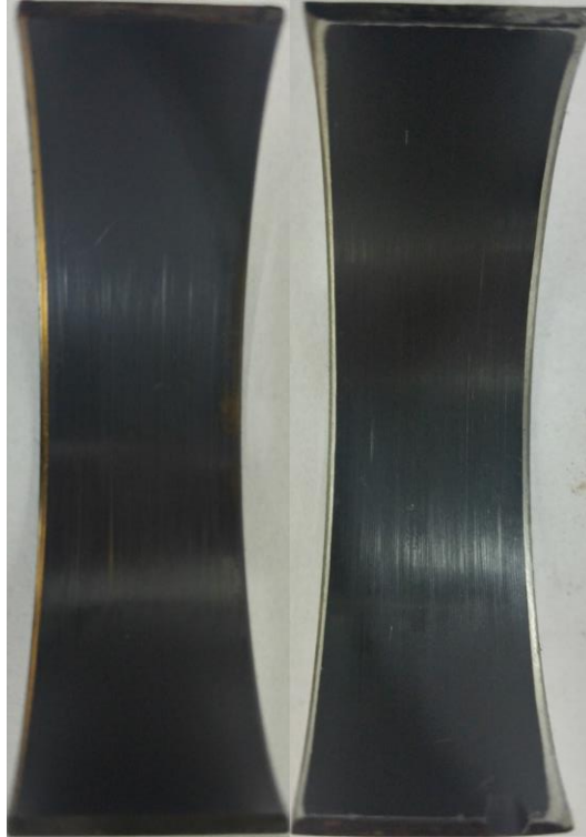
Fig.7 Tested bearings coated with K-340 wear resistant coating left – steel-bronze bearing, right – steel aluminum bearing
