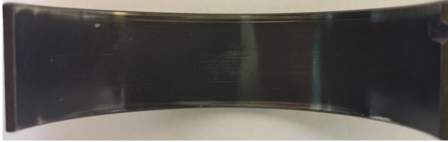
Fig.8 King aluminum alloy HP bearing coated with K-40 after direct friction test
